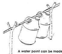
A water point can be made from 1½ gallon bleach bottles. Tip 'em to pour.
