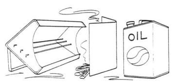
Reflector oven and windbreak from one 5-gallon tin.
