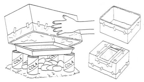
box oven over the pan. Make a small gap for air at each end of the oven by scraping some dirt away. Air circulation is needed to keep the charcoal burning.
